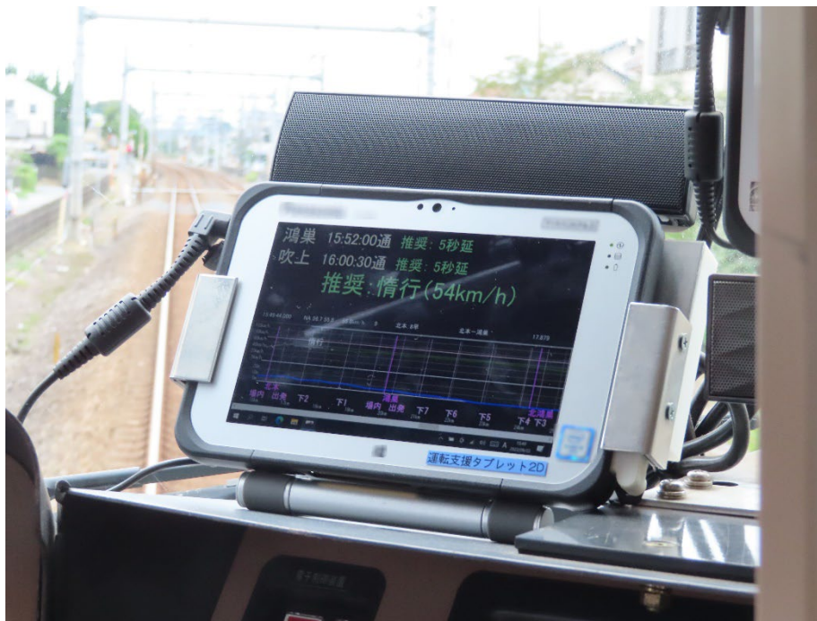
Fig. 1 Example of Driver Advisory System Installed on Driver’s Cab
