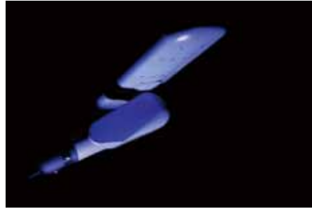
Measurement test of pressure distribution on pantograph-head with pressure sensitive paint in the large-scale wind tunnel
