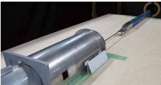
Experiments using a model train and a model tunnel with the same shapes and dimensional ratios as the real versions
