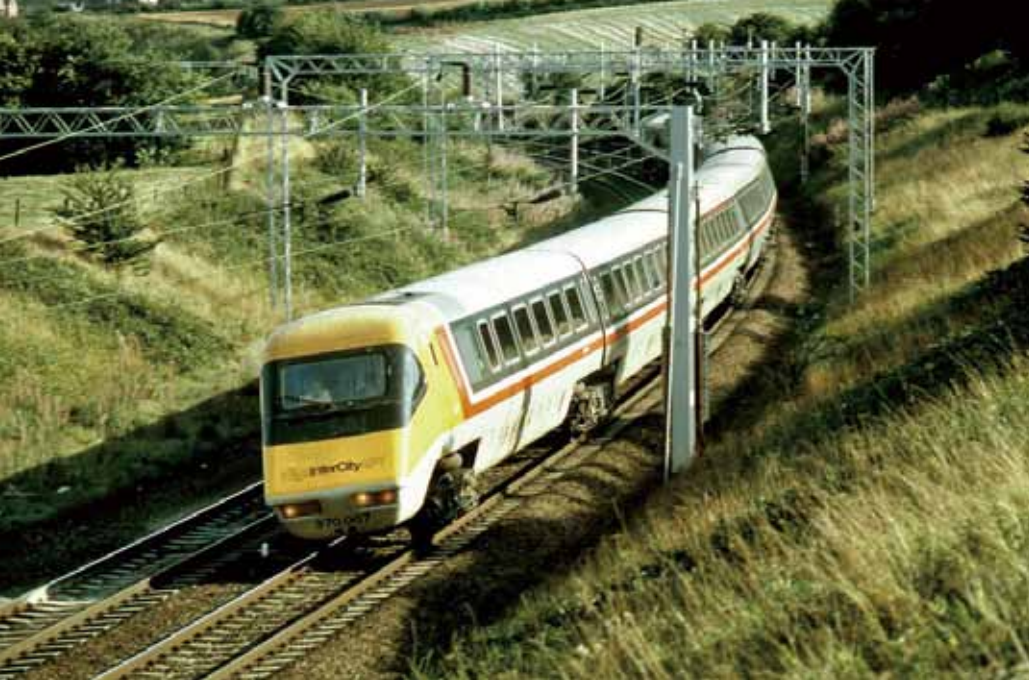
The Advance Passenger Train: an underfunded and over complex attempt to overcome the sinuous nature of old track by an sophisticated train.
