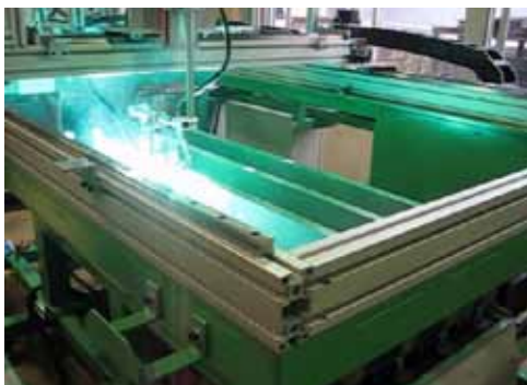
MIG welding by an automatic welding machine
