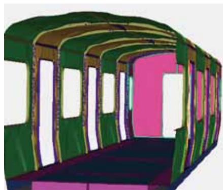
A light weight and less deformable body is realized with an integral structure of concavo-convex shapes shell by press forming.
