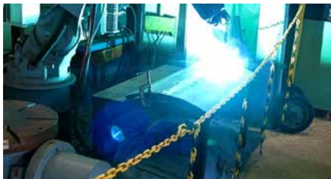
MIG welding of roof structure
