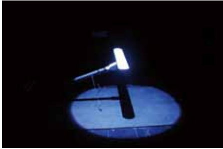
Measurement test of pressure distribution on pantograph-head with pressure sensitive paint in the large-scale wind tunnel
