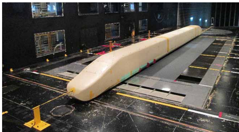
The track surface flow is simulated using a moving belt and a boundary layer suction device. A spire installed on the front vehicle controls the boundary layer formed under the vehicle floors to reproduce the underfloor flow field on the intermediate vehicle.
