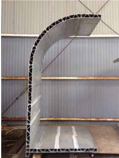
A scale model of half cross-section of double-skinned bodyshell made from a flame-resistant magnesium alloy
