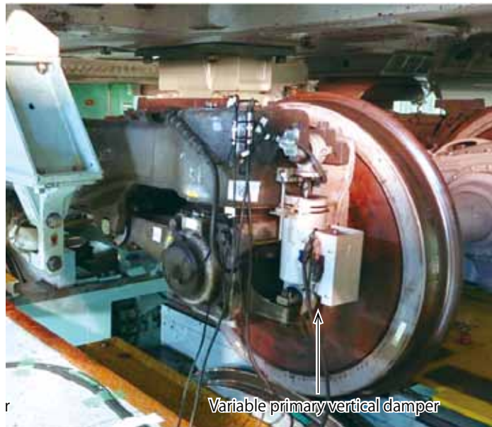
A prototype of vertical vibration damping system was tested on the rolling stock test plant in RTRI.
