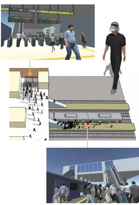
VR(Virtual Reality) simulation of walk-through in a station wearing a head mount display
