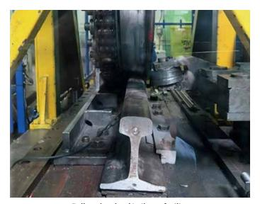
Full-scale wheel/rail test facility
