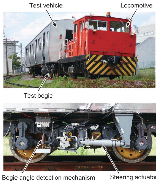
Fig. 8 Running test for steering performance evaluation
