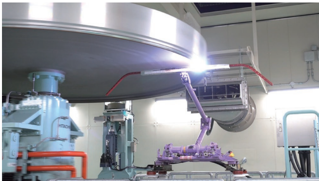
Fig. 4 Photo of energization test (light between disk and pantograph is an arc generated by contact loss)
