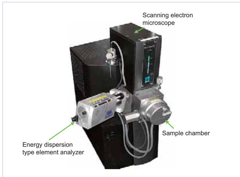
Fig. 3 Low-vacuum scanning electron microscope equipped with energy dispersion type element analysis function
