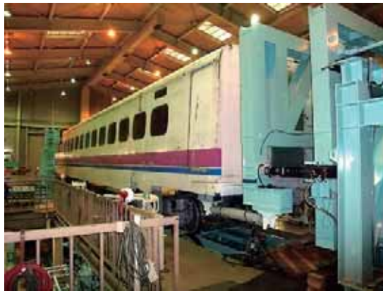
Fig.1 Vehicle-testing apparatus adding simulator for inter-carbody motion
