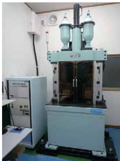
Fig. 2 High-speed material testing machine
