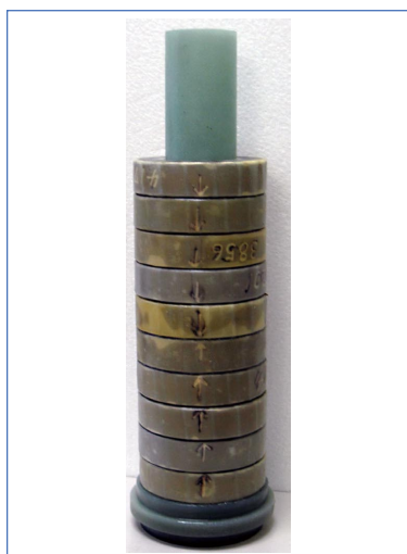
Fig. 1 A small superconducting magnet (outside diameter of superconducting bulk 80 mm, inside diameter 50 mm, 10 layers)
