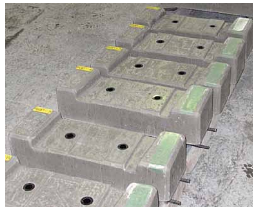
► Steel fiber reinforced geopolymer sleeper block (no rebars)
