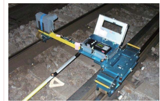
▶ Rail surface irregularity continuous measurement device
