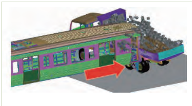
Fig.1 Example of train collision analysis (collision speed 54km/h)
