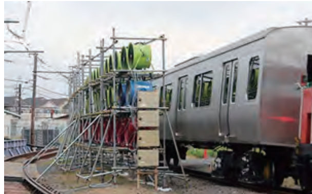
Fig 4-1-1 Image showing the cross wind running test
