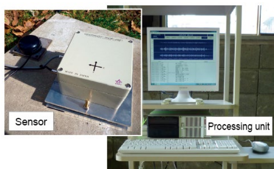
fig.1 Picture of prototype advanced seismograph for earthquake early warnings
