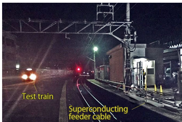
Fig. 4-8-1: Train running test using superconducting feeder cable
