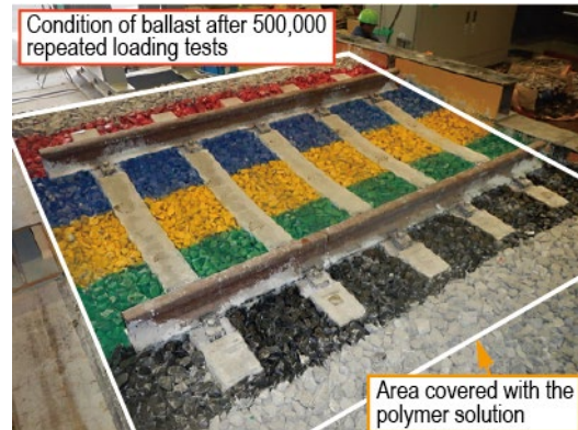
Fig 4 Confirmation of effectiveness of ballast migration countermeasure
