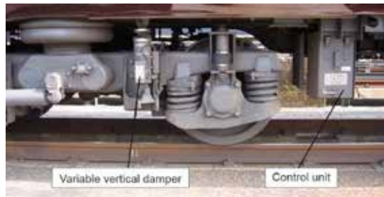
Vibration Suppression System Using Variable Vertical Dampers which suppresses vertical car body vibration and improves riding comfort
