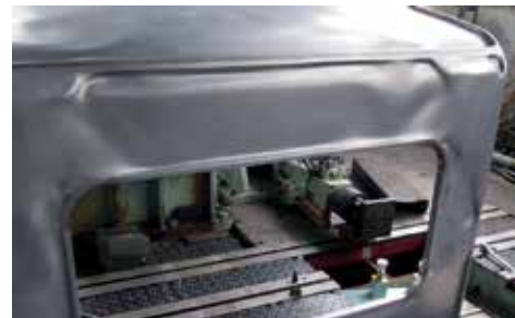
Fig. 2 Press-molded body structure
