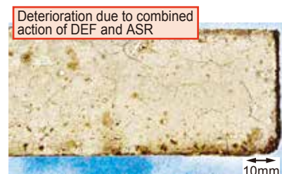
Fig. 2 Effect of ASR on DEF expansion (under unfavourable conditions)
