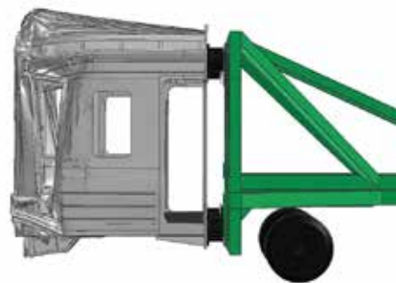
Fig. 3 FE result of deformed shape of test vehicle. FE result agrees well with test result.
