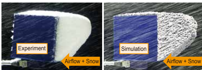
Fig. 2 Comparison for a cubic model between the snow accretion experiment and simulation
