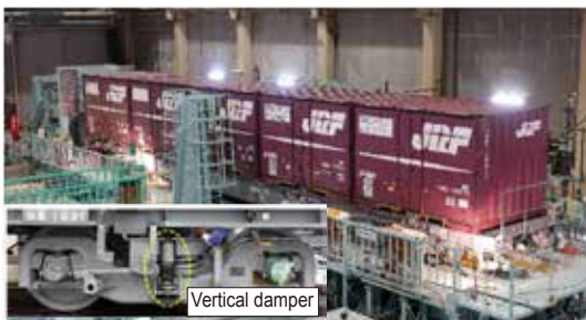
Fig. 2 Vibration tests on rolling stock test plant
