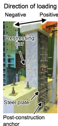
Fig. 3 Effect of reinforcement for proof strength improvement
