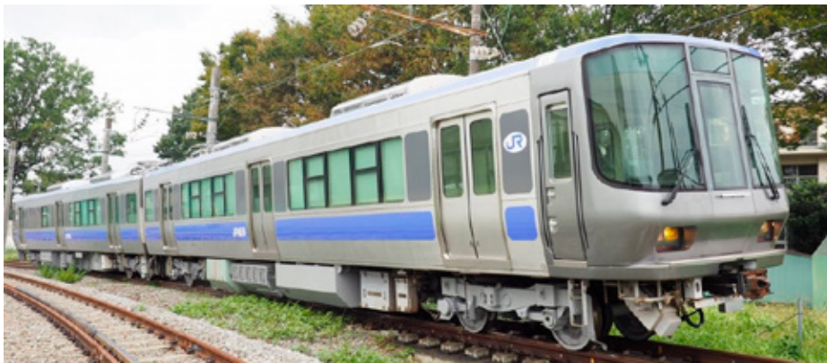
Fig.1: Fuel cell hybrid powered test railway vehicle
