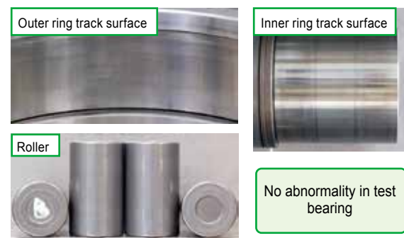
Fig. 3 Test bearing after bench test (equiv. of 800,000 km)
