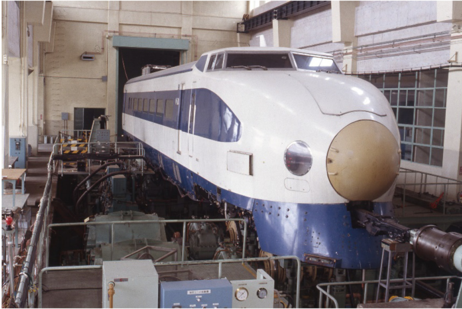
Fig.2 Sanyo Shinkansen test vehicle tested on this facility
