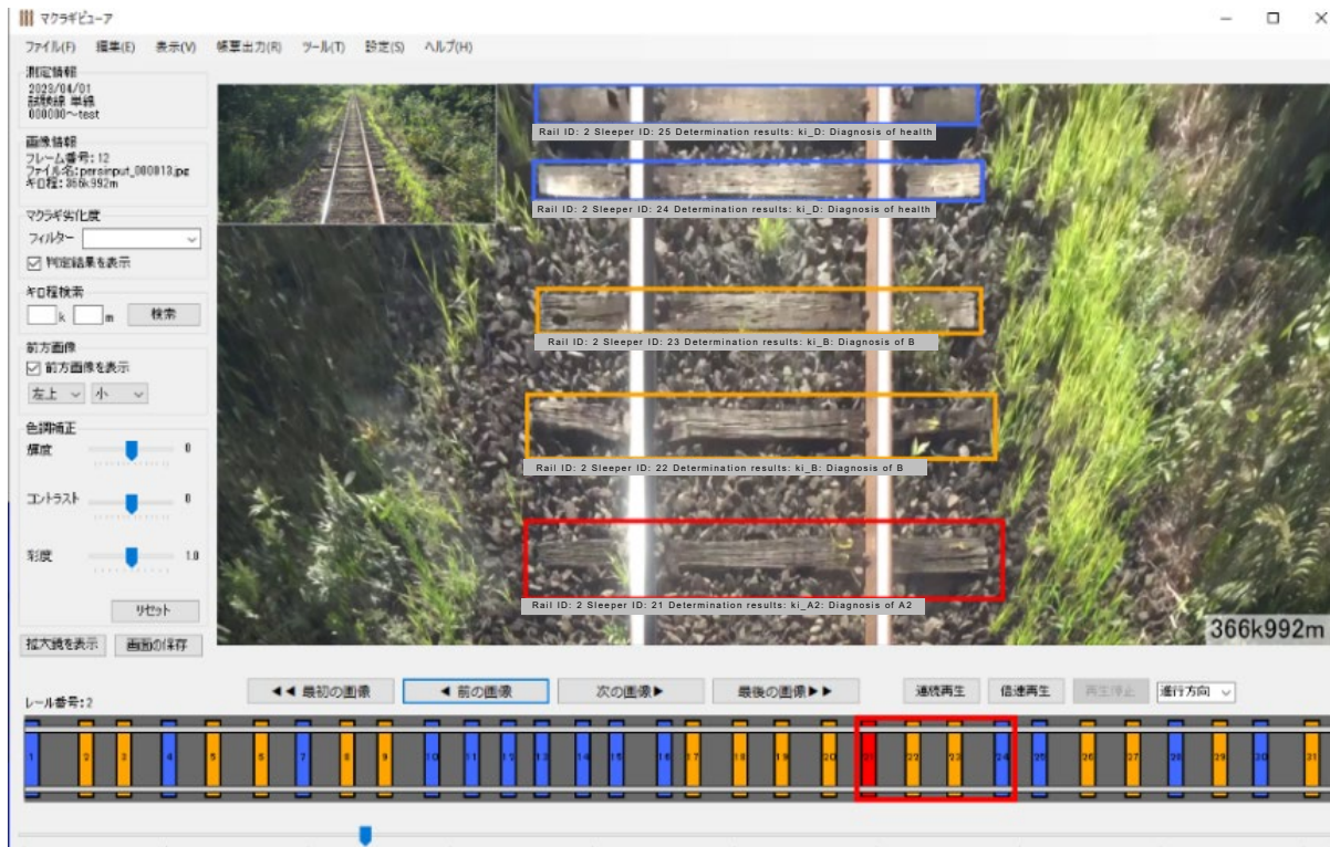
Fig. 4 Screen displaying determination results obtained from the Sleeper Viewer
