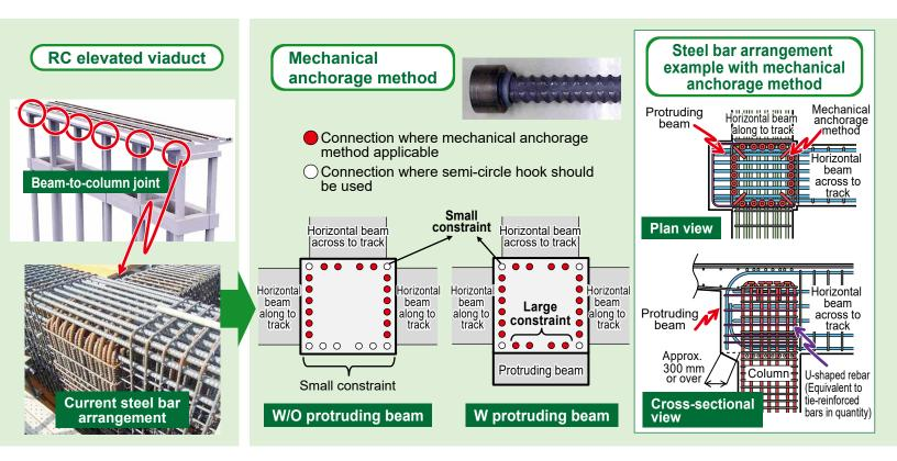
Mechanical anchorage method for the beam-to-column joint of RC viaducts
