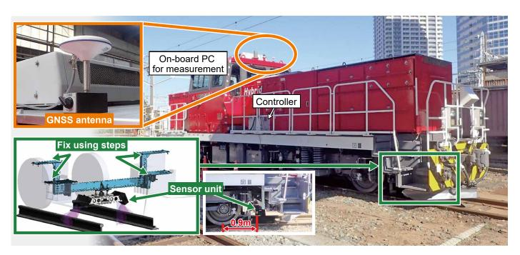
Dynamic track measuring device for gauge and twist
