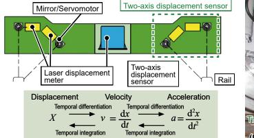
(a) Measuring principle of inertial mid-chord offset method
