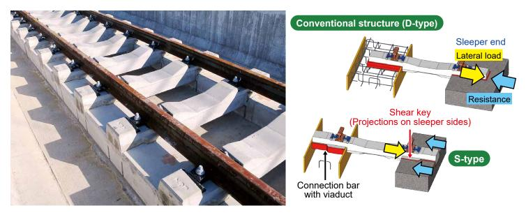
Solid-bed track equipped with resilient sleepers using the shear-key
