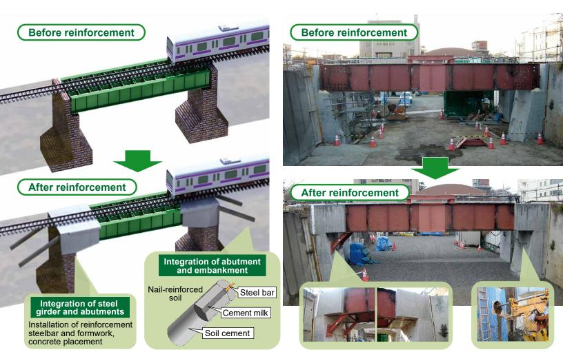
Seismic reinforcement technology of steel railway bridges (Integration of bridge girder, abutment, and embankment)
