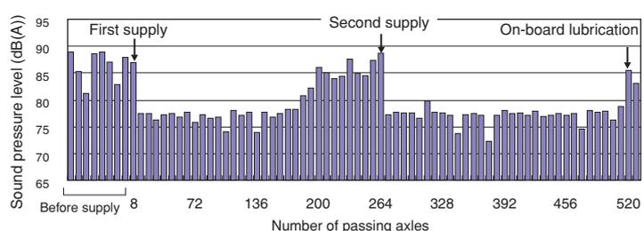
**Fig. 4** Effect of the friction moderator in reducing rolling noise, measured at 2.1 m from center of track gauge
