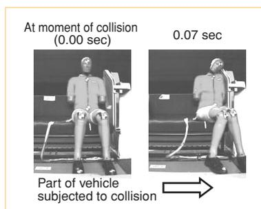
**Fig. 2** Collision experiment with panel divider
