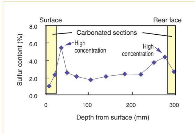
**Fig. 3** Distribution of sulfur within typical concrete sample
