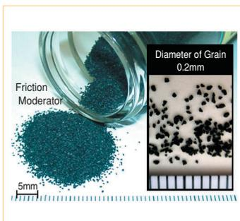
**Fig. 2** Grain diameter
