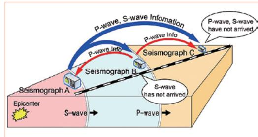
Fig. 2 Seismograph two-way communication after detection of the P-wave
