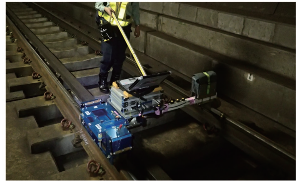
Fig. 6 Measurement with rail surface roughness continuous measurement trolley
