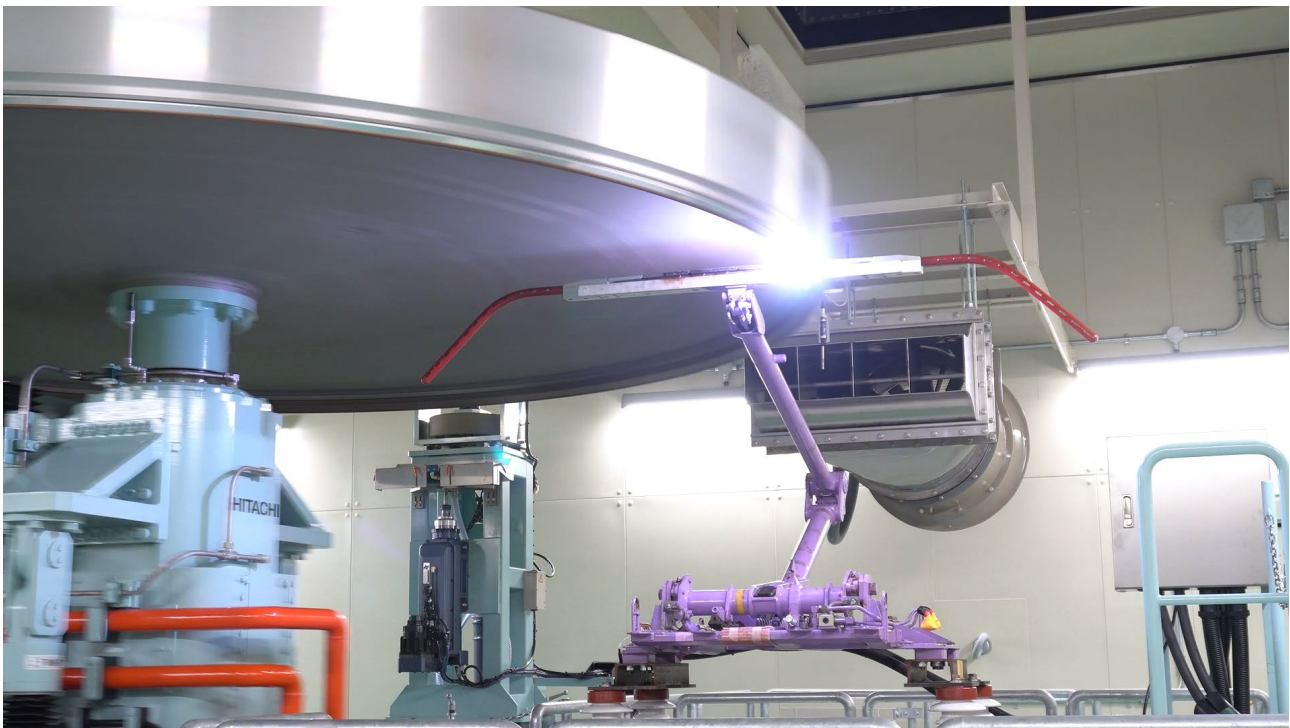
Fig.2: Testing on the high-speed test facility for pantograph/OCL systems (Rotating speed: 360 km/h, AC200V, 600A)
