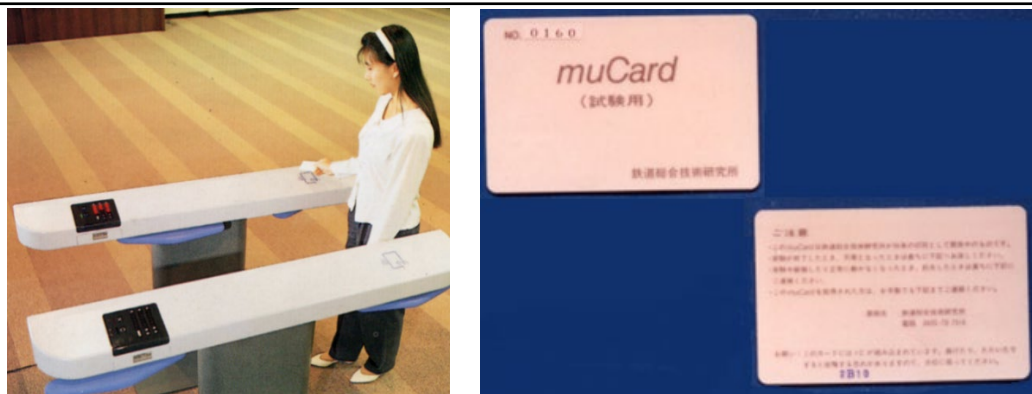
Fig. 1 Prototype Automatic Fare Collection Gate and Prototype Contactless Smart Cards
