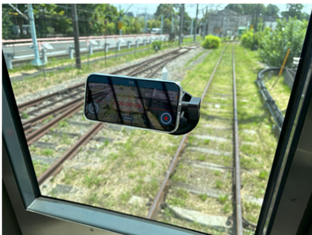
Figure 2: Example installation of a smartphone in a revenue train cab (mounted using a suction-cup fixture)
