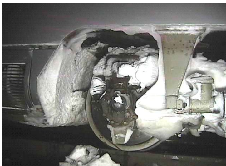
Fig. 1 Snow accretion found on an actual vehicle
