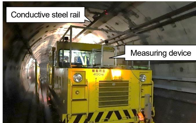
Fig. 4 Measurement of the conductor rail of the Toei Oedo line
