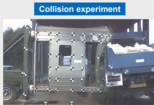
(b) Experiment between a railway vehicle and a dump truck and analysis of the results
