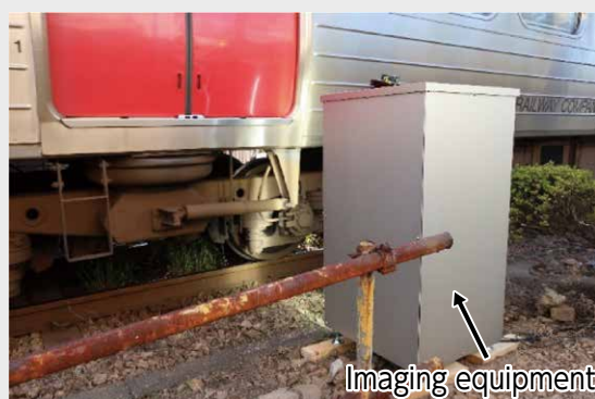
(b) Imaging equipment capturing a passing vehicle
