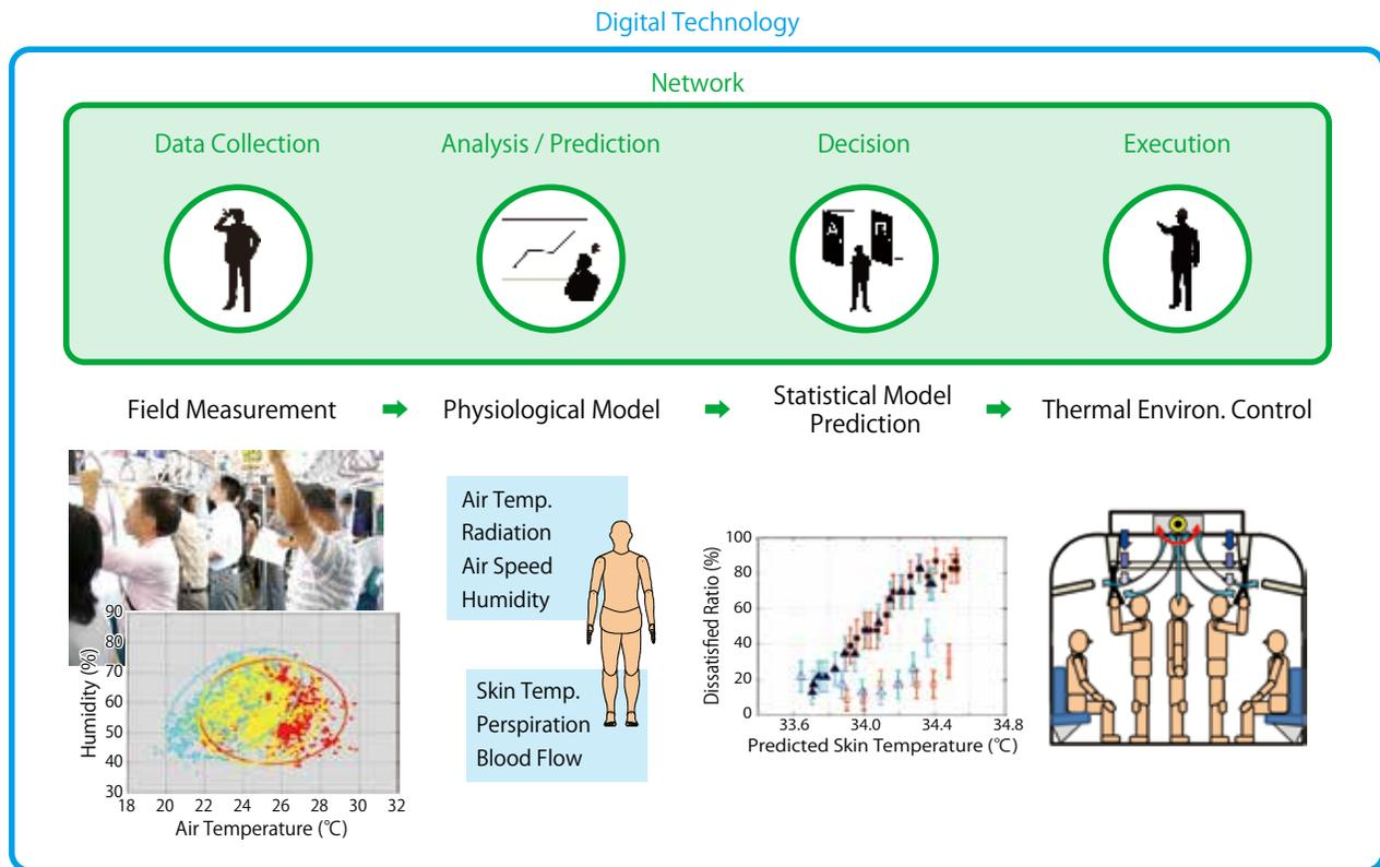
An example of utilizing digital technology for the control of thermal comfort
