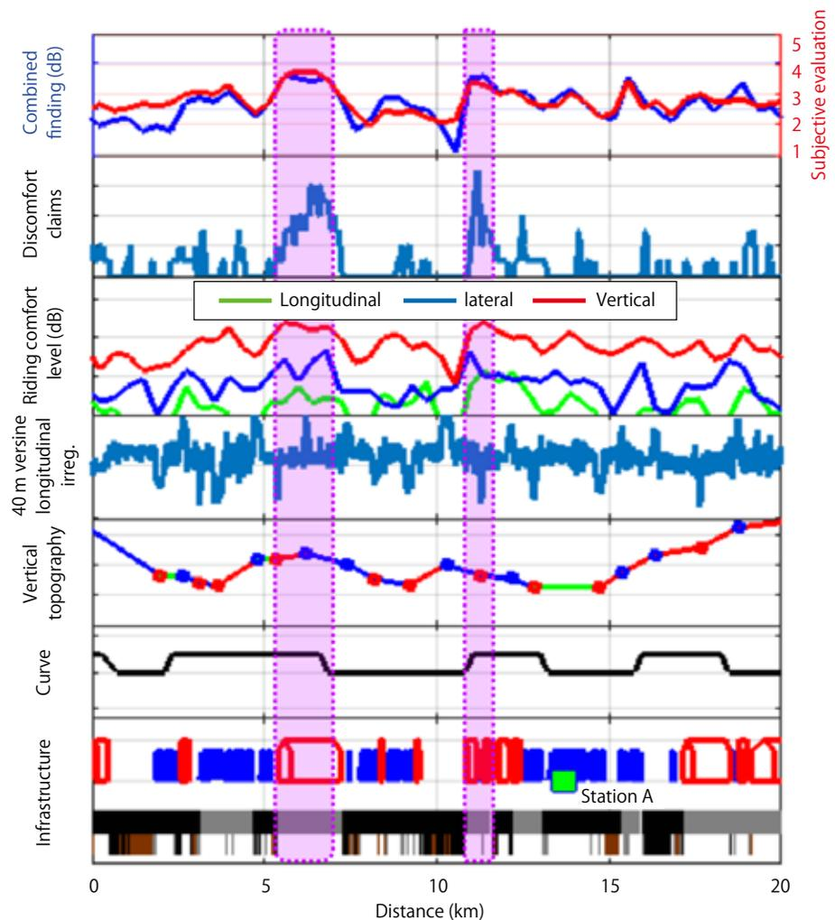
**Displaying along distance structure of track, infrastructure and vehicle vibration data reflecting the human perception sensitivity to vibration, the causes for the vibrations can be multilaterally identified and analyzed. The combined findings estimating the sensory ride comfort, obtained by synthesizing the measured vertical, lateral, and longitudinal accelerations are in good agreement with the bodily sensation assessment in an experiment.**
