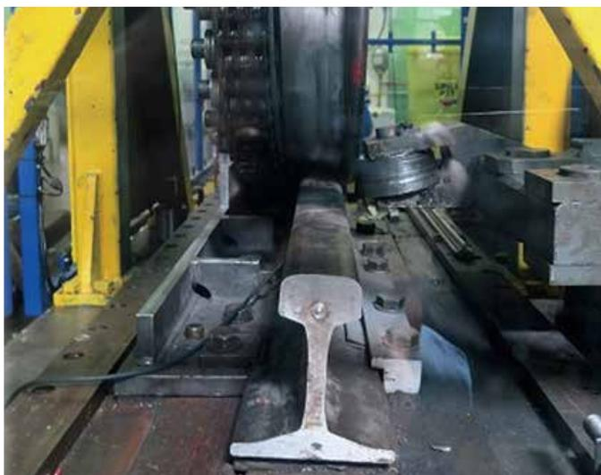
**Full-scale wheel/rail test facility**
