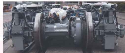
Figure 5. Gauge-changeable truck (type B).
