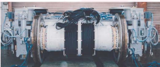
Figure 3. Gauge-changeable truck (type A).
