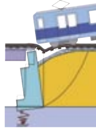
Figure 1. Image of the damaged bridge abutment at earthquake.
