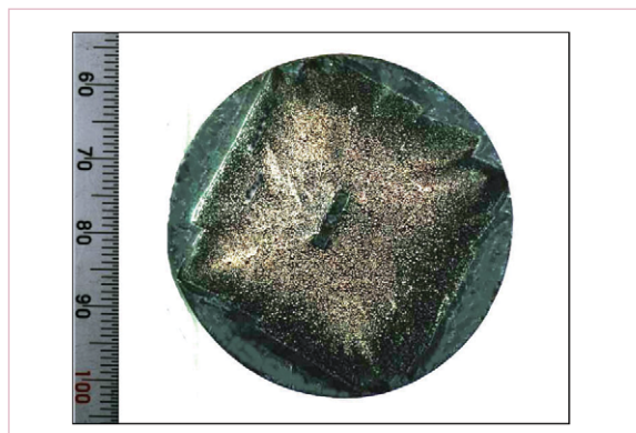
Figure 2. Photograph of the surface of our Ag-added Y-based high-temperature superconducting bulk (maximum heat treatment temperature: 1,060 °C, undercooling temperature: 10 °C).
