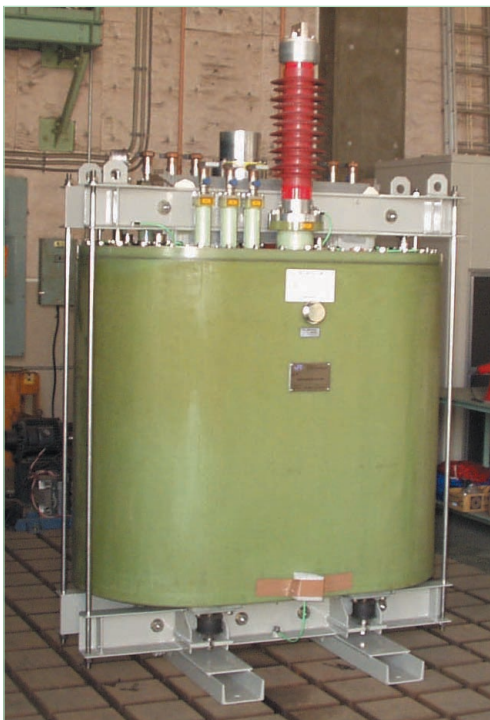
Figure 1. Appearance of the test-manufactured superconducting main transformer
