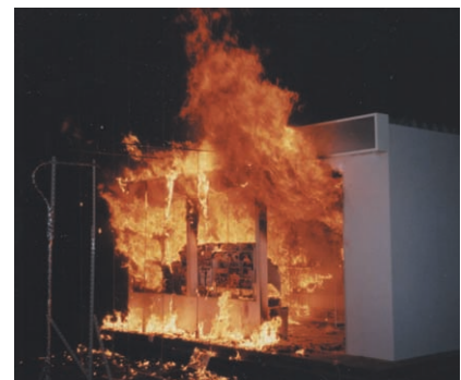
Figure 3. Combustion experiment using full-scale model of kiosk
