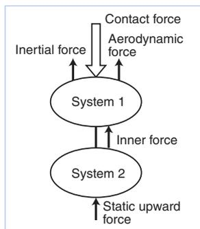
**Figure 1.** Forces acting on a pantograph
