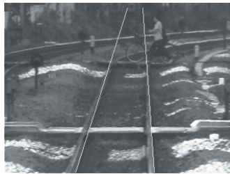
Figure 1. Extraction of rails through application of the Hough transformation
