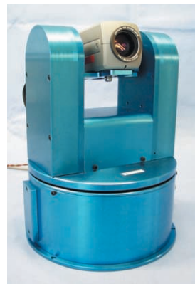
Figure 3. Pan head for automatically tracking rail vanishing point
