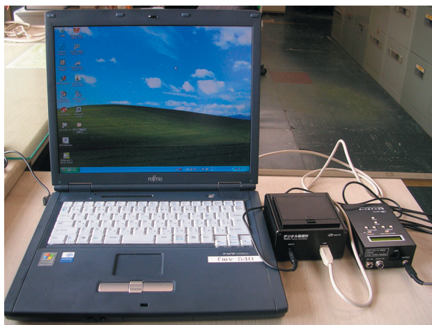
Fig. 1 Component parts of the ride comfort evaluation system
