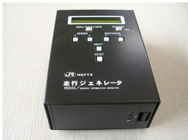
Fig. 3 Running motion data generator
