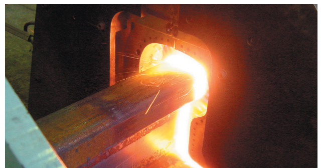
Fig. 4 Gas pressure welding test using an oxygen/hydrogen flame for rail welding
