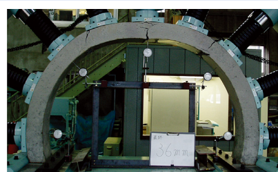
Photo 2 State of cracking and deformation (at final push-in)
