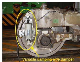
Fig. 2 Installation of variable damping axle damper
