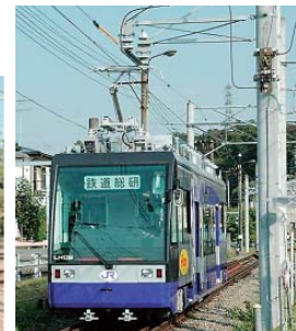
Fig. 4 Quick charging from rigid contact wires
