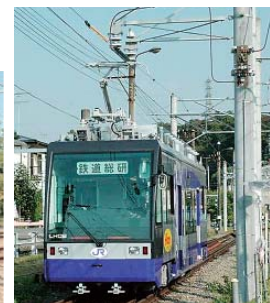
Fig. 4 Quick charging from rigid contact wires
