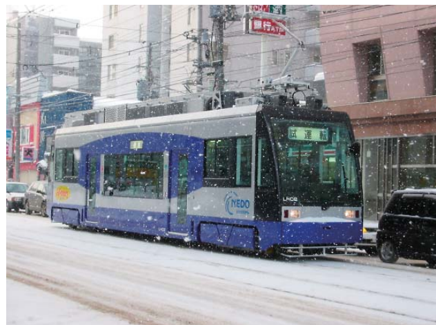
Fig. 2 The Hi-tram under a running test in snowy conditions in Sapporo
