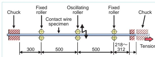
Fig. 3 Contact wire fatigue test device
