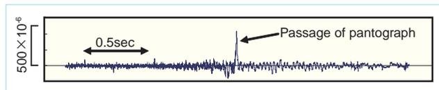
Fig. 2 A strain waveform in a contact wire
