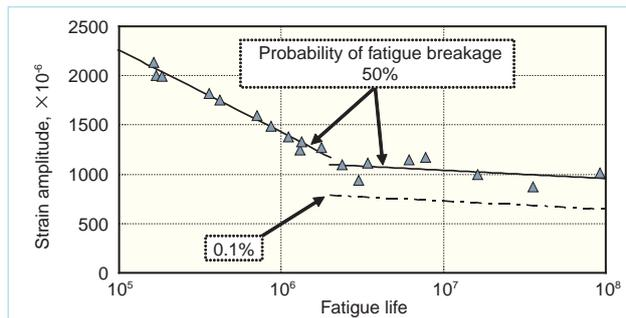
Fig. 5 Approximation of fatigue life property of SN-W contact wire
