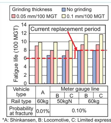
Fig. 5 Example of evaluated fatigue life of CWR
