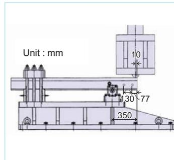
Fig. 2 Bending fatigue test of fish-plated joint rail
