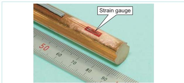
Fig. 1 A strain gauge fixed to a contact wire
