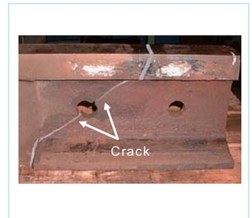
Fig. 3 Example of rail broken in fatigue test
