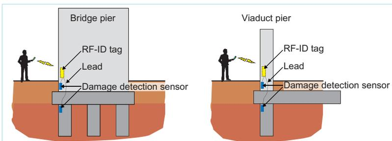
Fig. 3 Installation of damage detection sensors
