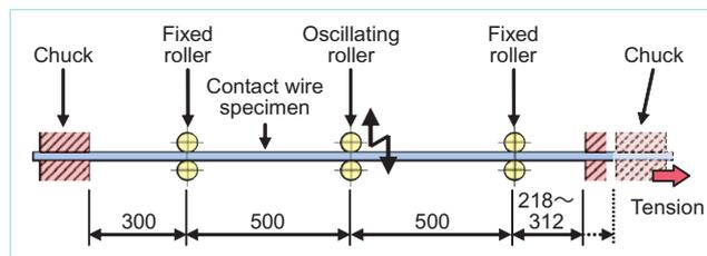
Fig. 3 Contact wire fatigue test device
