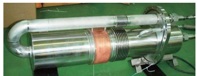
Fig. 3 Practical version of a pulse-tube cryocooler for a traction transformer
