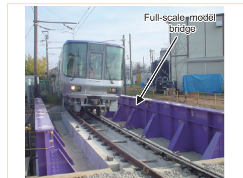
Fig.2 Full-scale model bridge
