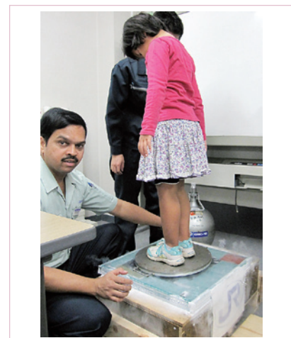
Fig. 4. Levitation of child using a repulsive force between home made batch processed LRE-123 pellets and home made permanent magnet disk
