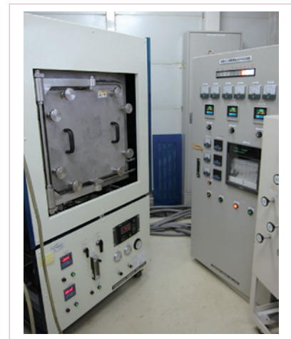
Fig. 1. Furnace designed for batch production of LRE-123
