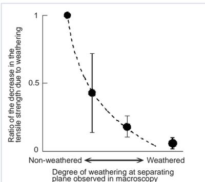
Fig. 3 Degree of the decrease in the tensile strength due to weathering
