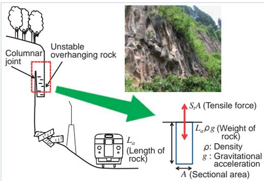
Fig. 1 Schematic diagram and a photograph of unstable rock on slope
