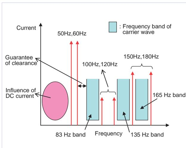
Fig. 1 Frequency band versus power source harmonic noise
