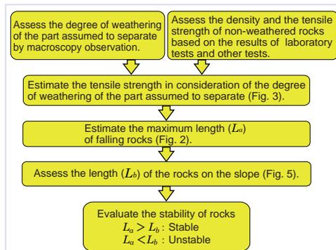
Fig. 4 Flow chart showing the process needed to evaluate the stability of rocks
