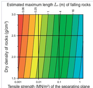
Fig. 2 Nomogram for the estimation of maximum length of the falling rock
