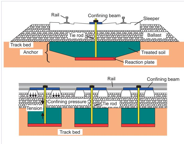
Fig. 1 Basic structure of the Prestressed Ballast Track
