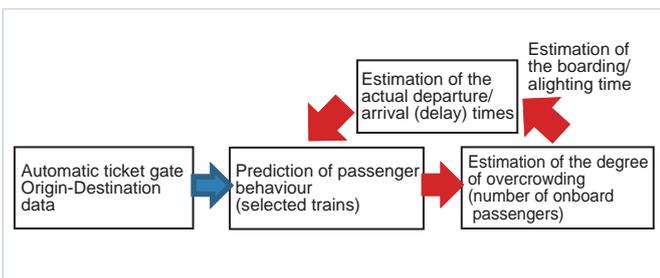
Fig. 1 Flow of simulation
