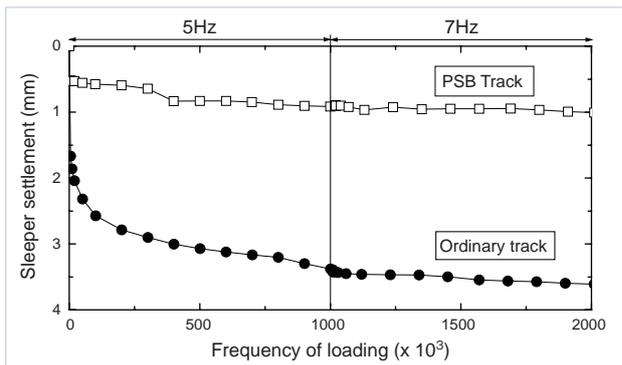
Fig. 2 Results of a repeated loading test on PSB Track (axle load 160 kN)
