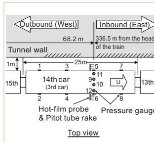
Fig. 1 Layout of equipment on the train travelling through a double-track tunnel
