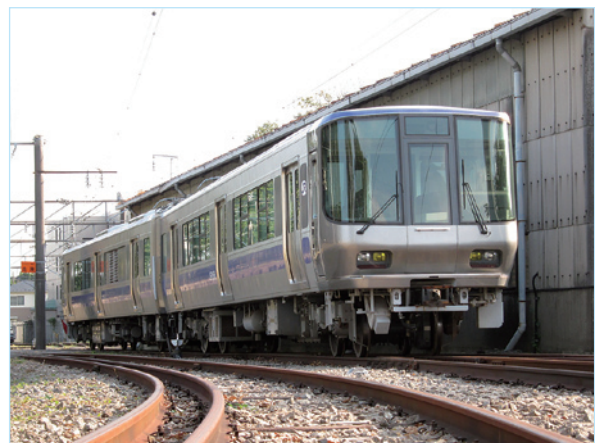
Fig. 3 Hybrid railway test vehicles with fuel cells and batteries
