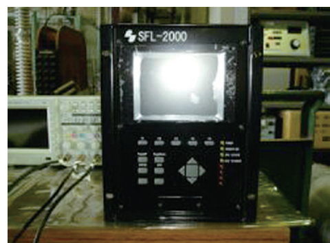
Fig. 3 Prototype surge detection type fault locating system (waveform processing device)
