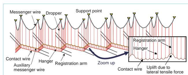
Fig. 2 Calculated static structure of compound catenary system
