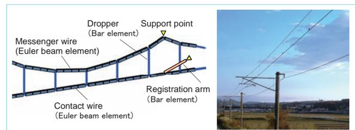
Fig. 1 FEM model of catenary system
