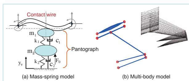
Fig. 4 Pantograph model
